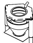
4.7.0: Material Discharge Module with inner tube, air filter and passive (manual) covering
