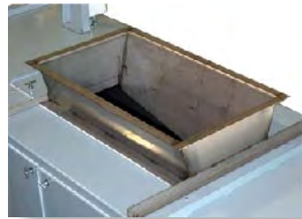
Special inlet configurations to promote material flow and reduce motor HP
