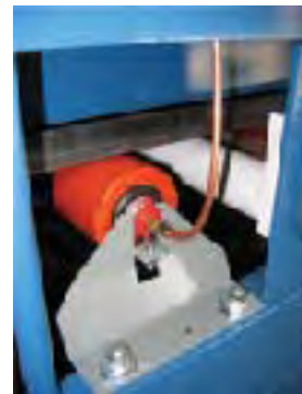
Optional pulley and idler lubrication manifold mounted external to the enclosure
