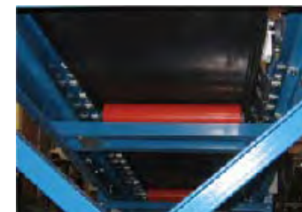
Standard slack belt support idler
