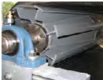
Optional Winged Tail Pulley prevents material build-up
