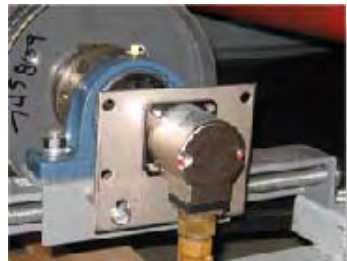
Speed sensing is digital and accurate over an infinite speed range.
