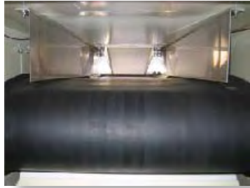
Full length adjustable skirt boards
