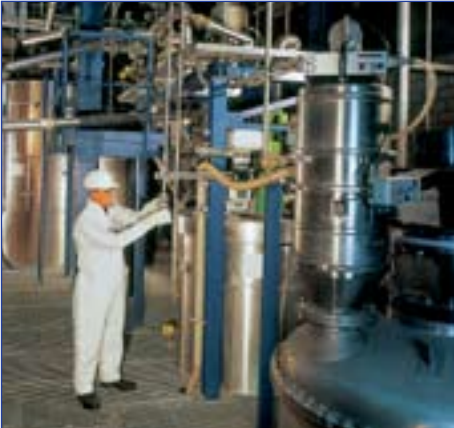
Transfer of metal powders with bulk densities up to max. 10 kg/dm 3 with Vacuum Conveyor.
