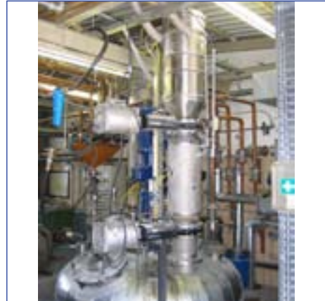
Conveying of dye pigments. Loading of a stirring vessel with a double-valve INEX powder lock under a VR450.
