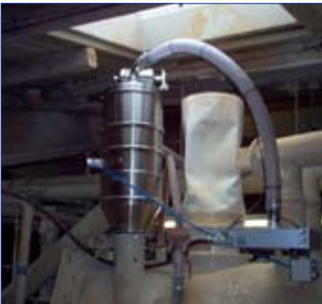
Conveying of construction materials and additives with a VR450 and with an external Vacuum Pump.
