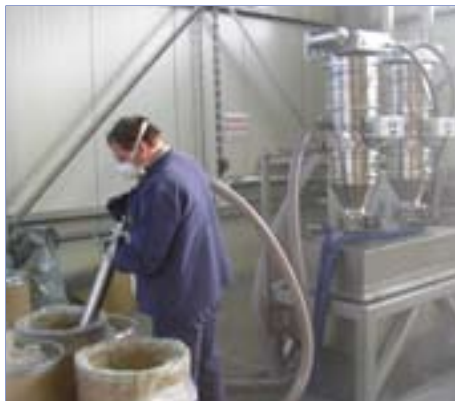
Discharging of drums with inliner by manual suction lance. Transport of chemical powders with two VR315.
