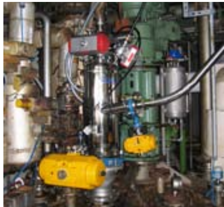
Powder Transfer with a 10 bar pressure rated INEX (Inert) Vacuum Conveyor into a pressurised reactor.
