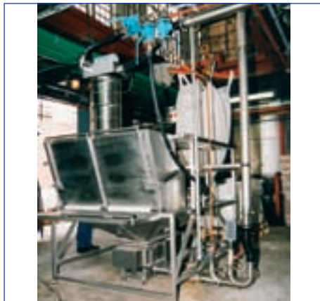
Big-Bag and Sack-unloading station with lump breaker. Feeding of resins and chemicals into the Vacuum Conveying line.
