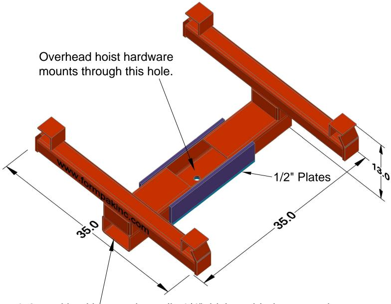
4x6 steel backbone, tube walls 1/4" thick, welded construction.
