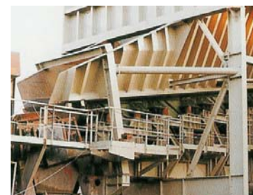
Extrovib discharge system for truck and rail dump stations
