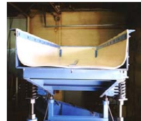
Replaceable, rubber liner prevents build-up of sticky coal
