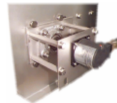
Digital Pulser Mounted To Tail Pulley
