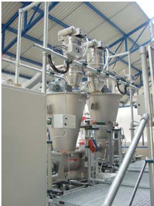
A pair of Volkmann Conveyors supplying material to metering feeders.
