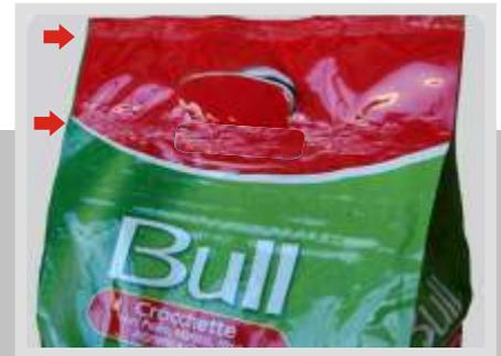
■ Single or double heat-sealing of bags at different heights on the bag face, fully programmable
